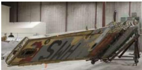
*The starboard end of the one-piece wing.*
