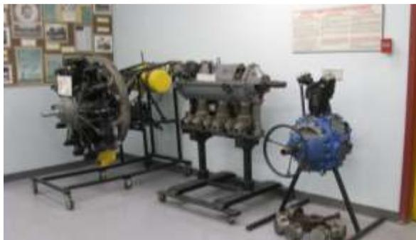
*Engines (L-R): a Jacobs L6MB, Fairchild Ranger cut-a-way, and a partial Jacobs showing its internal workings.*
