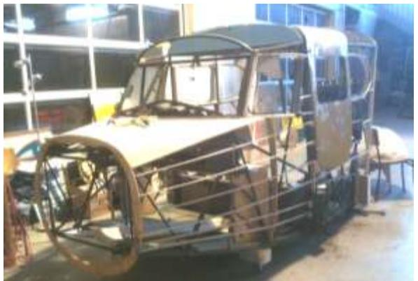
*The second "simulator-to-be" as it looked in early April, nearly ready for the application of fabric covering. It will house a computer with the "Flight Simulator" program c/w wartime aircraft.*
